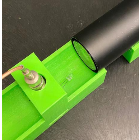
Fig. 1. PMT HRNG Experimental Setup. A 3D printed holder houses the PMT and LED in the dark box (not shown).
